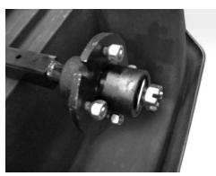
Place the hub assembly, spindle washer, and spindle nut on the end of the axel as pictured. Tighten the spindle nut until the hub bearing and washer are tight against the back of the axel, the rotation of the hub should be difficult. Loosen off the nut 1/4 - 1/2 a turn so that the hole in the axel is centered between two of the notches in the spindle nut.
