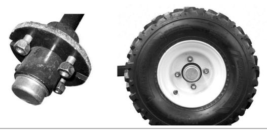
Place dust cap on hub. Using a rubber mallet, tap into place. Finally remove the hub nuts and place tire and rim onto the hub so the valve stem is facing out and tighten tire onto hub. Repeat for the other side.
