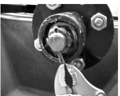
Insert and bend sides of cotter pin to lock the nut in place.
